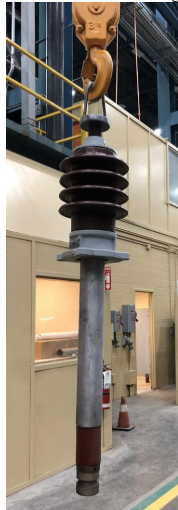
Fig 6 – Lift bushing with lifting eye.
