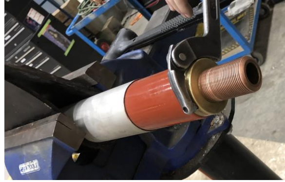
Fig 15 – Base of the bushing core
