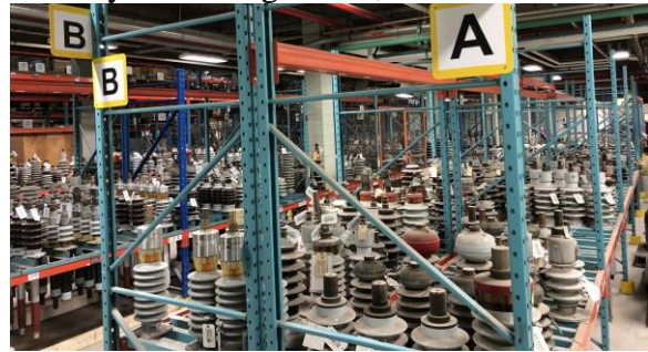
Fig 1 – Spare bushings at Hydro One Central Maintenance Services.
