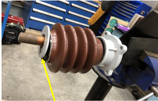
Fig 9 - Bevelled washer
