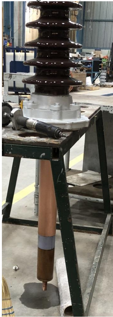
Fig 4 – Visually inspect for damage or oil leaking.
