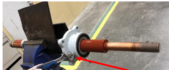
Fig 10 - Remove ground continuity screw
