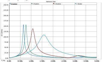
Figure 1 Frequency Scan of the Wind Farm Collector System
