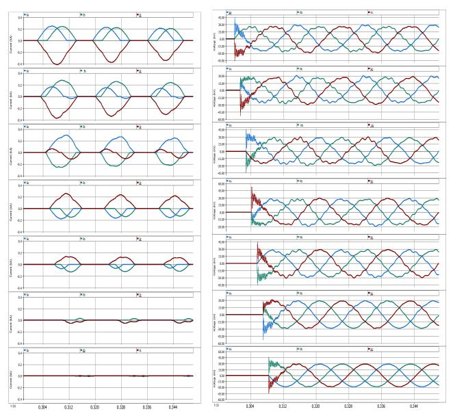
Figure 4 Transformer Inrush Current for Various Switching Points and Transient Voltage at Transformer Terminals for Various Switching Points
