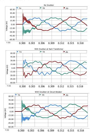
Figure 3 Impact of Installation of RC Snubber Circuits on Voltage Transients at Transformer Terminals
