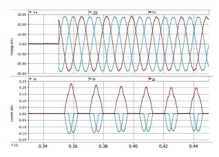
Figure 2 Voltage and Current Waveforms of an Energized Transformer
