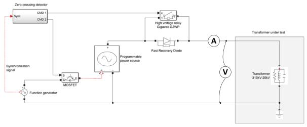
Figure 1: Schematic of the TRV test setup
