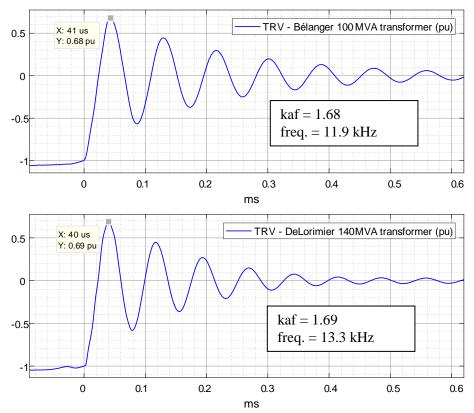
Figure 2: Transformer-fed fault TRV measurements
