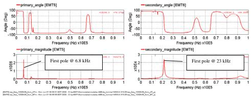
Figure 4: frequency response from manufacturer model for De Lorimier transformer
