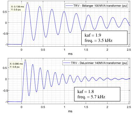
Figure 3: Transformer-secondary fault TRV measurements
