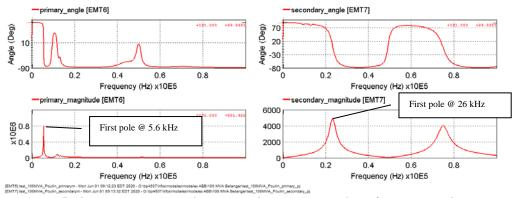
Figure 5 : frequency response from manufacturer model for Bélanger transformer
