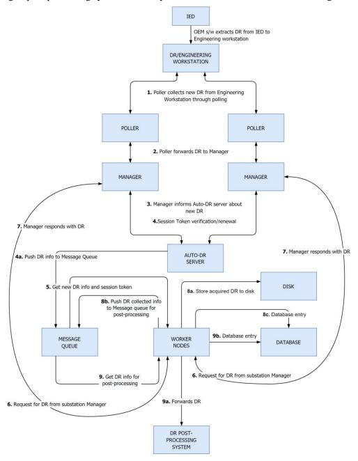
Figure 2. Detailed workflow of Auto-DR architecture
