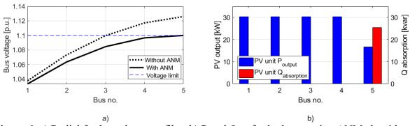
Figure 6: a) Radial feeder voltage profiles, b) P and Q at feeder buses using ANM algorithm.
