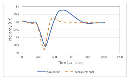
Fig. 8. Simulation and measurements for PV plant disconnection.
