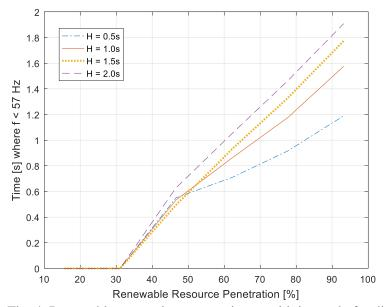
Fig. 4. Renewable generation penetration sensitivity study for different inertia constant values.
