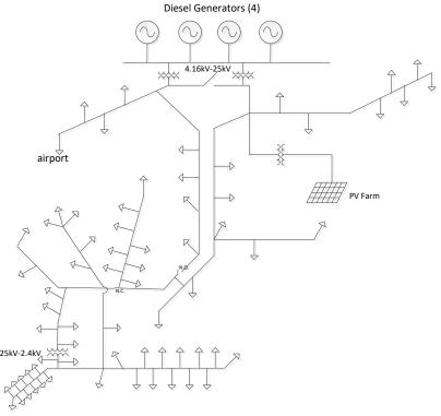
Fig. 7. Simplified electrical system topology.
