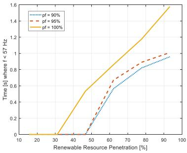
Fig. 6. Renewable generation penetration sensitivity study for different load power factor values.
