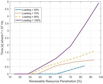
Fig. 5. Renewable generation penetration sensitivity study for diesel generator loading factors.
