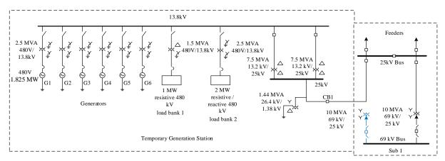
Figure 5: Single line diagram of the temporary generating station set up
