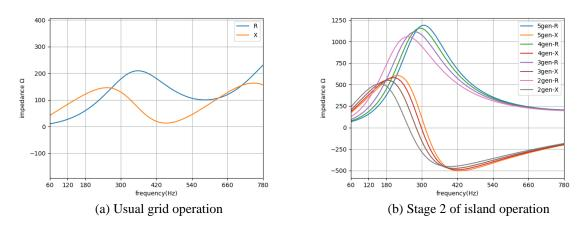
Figure 8: Frequency scan results at 69 kV bus at Sub 2
