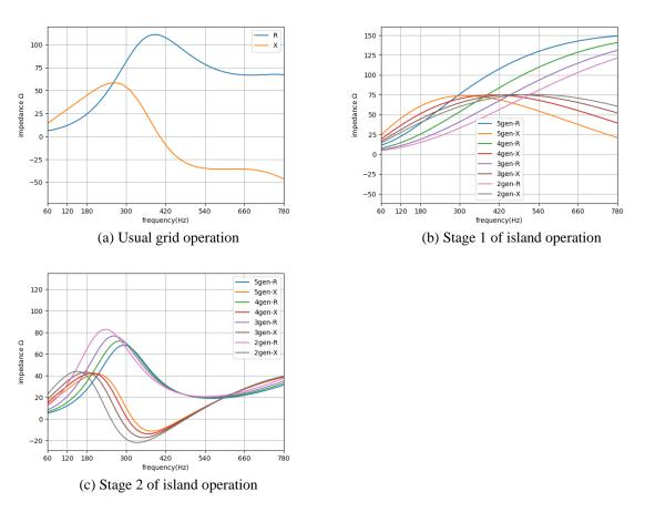
Figure 6: Frequency scan results at 25 kV bus at Sub 1
