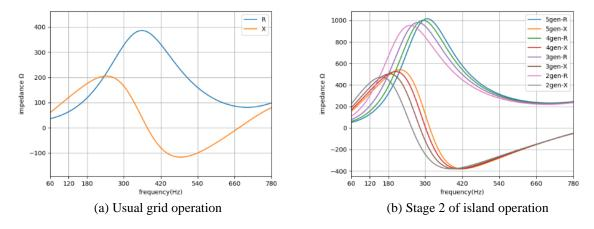
Figure 7: Frequency scan results at 69 kV bus at Sub 1
