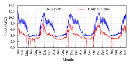
Figure 2: Historical maximum and minimum load for Sub 1, Sub 2 and 69 kV line 1 taps
