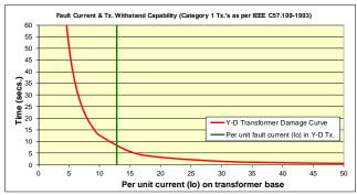
Fig. 3. Grounding transformer damage curve and fault contribution
