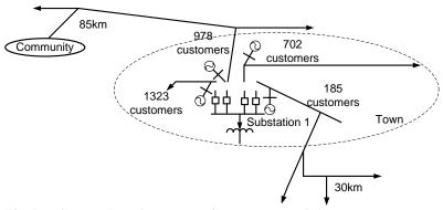
Fig. 5. Substation 1 Configuration and Generation Deployment
