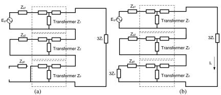
Fig. 2. Sequence network of a single-phase load supply, (a) Y generator and Yg- $\Delta$  transformer, (b) Yg generator and YgYg transformer
