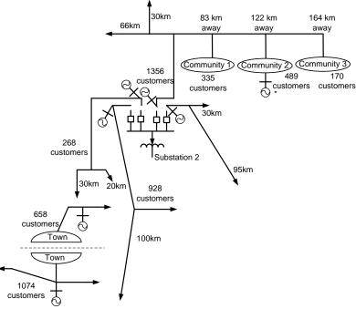
Fig. 6. Substation 2 Configuration and Generator Placement
