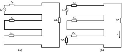
Fig. 1. Sequence network of a generator supplying a single-phase load, (a) Y generator (b) Yg generator
