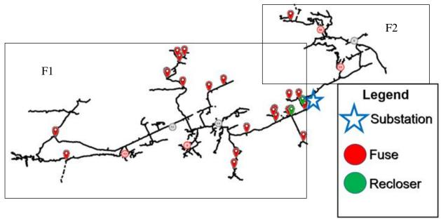
Figure 2 Simplified single line diagram of the feeder showing boundaries of the individual circuits.
