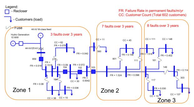
Figure 3 Simplified single-line diagram of circuit F2 with failure rates and customer count.
