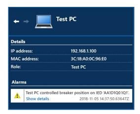
Figure 4. Alarm details: Test PC attempting unauthorized control of circuit breaker
