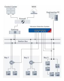
Figure 2. Connection of IDS to the substation network
