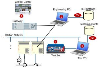
Figure 1. Attack vectors of a Substation
