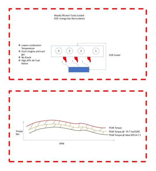
AFR stands for air to fuel ratio. Fuel doesn't burn on its own. It has to be mixed with air. AFR tells you how many parts of air are mixed with each part of fuel. For example, a 14.7:1 **AFR** (or just 14.7) means the mixture is 14.7 parts air to one part fuel
