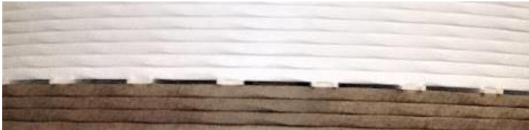
Figure 1 – Winding with a combination of high temperature Nomex® aramid wire insulation and thermally upgraded cellulose paper (photo: Siemens)
