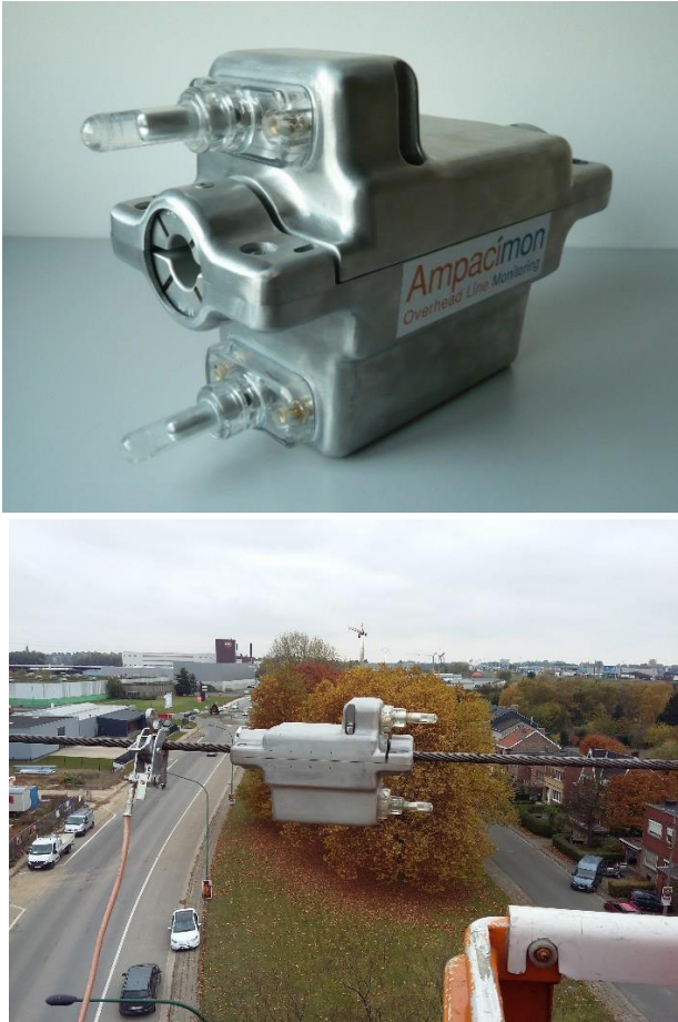
Fig. 1: Ampacimon™ vibration-based sensor [9]. (top) sensor at rest on a table and (bottom) sensor installed on a single conductor (picture taken during installation).
