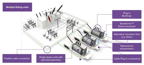
Figure 1 - Schematic arrangement of Siemens Energy's resilience concept [2]
